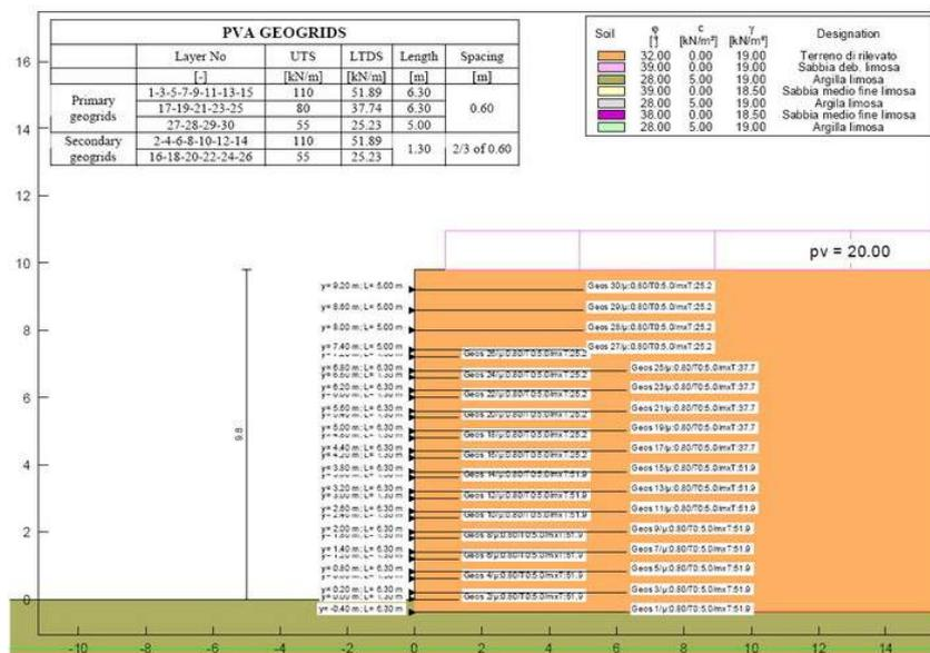
Figure 6. Cross section of the segmental retaining wall 10,2 m high
