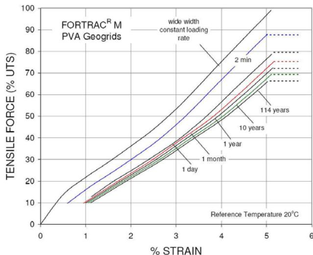
**Figure 5.** Isochronous stress-strain curves for the Fortrac® M PVA Product Line
