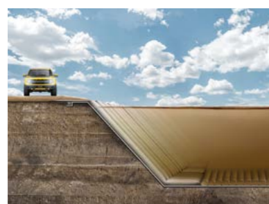
Geosynthetic Flexible Ballast Layer
