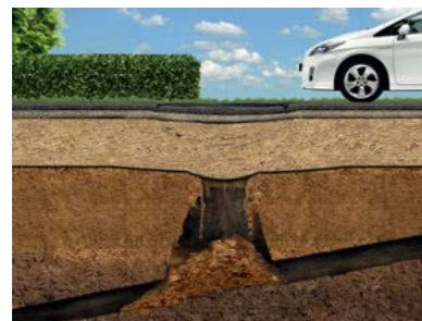
Bridging of Sinkholes
