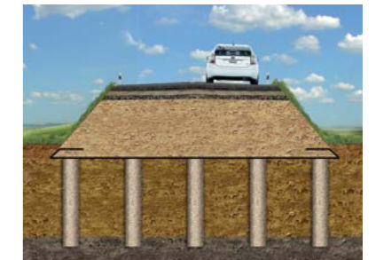
Geotextile Encased Columns (GEC)
