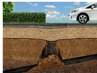
Bridging of Sinkholes
