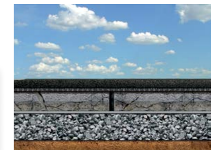
Rehabilitation of Concrete Pavements with Asphalt
