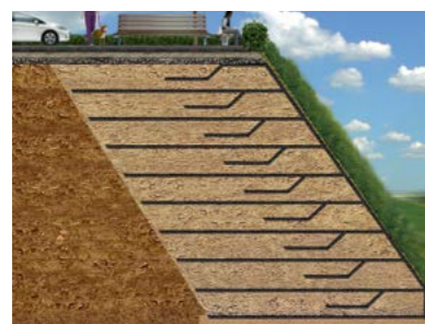
Geosynthetic Reinforced Soil
