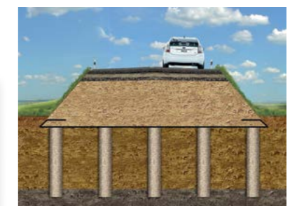
Geotextile Encased Columns
