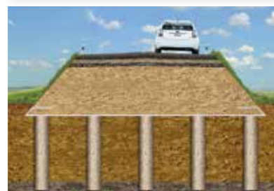
Geotextile Encased Columns (GEC)
