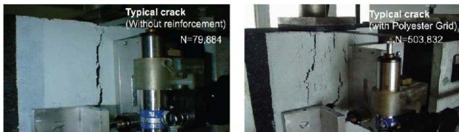
Figure 5.b – Comparison of cracks with and without reinforcement and the number of cycles conducted before the cracks reached the surface (Montestruque, 2002)
