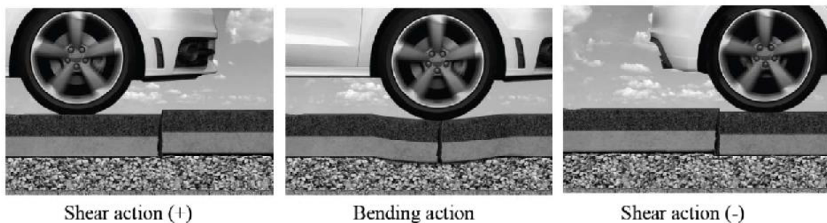
Figure 3 – Critical loading cases in a pavement crack
