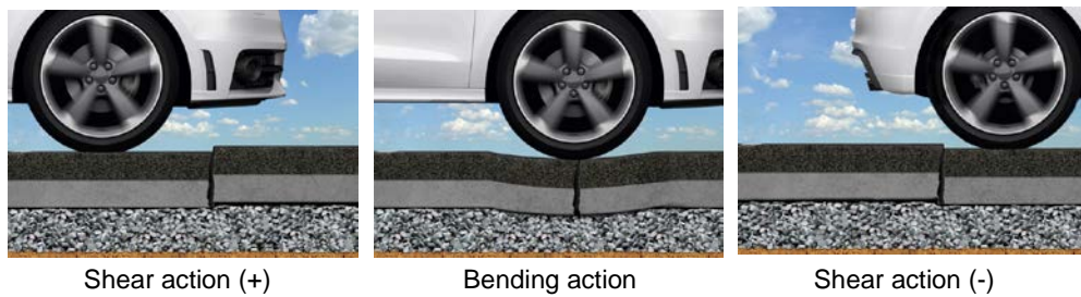
Figure 1. Critical loading cases in a pavement crack
