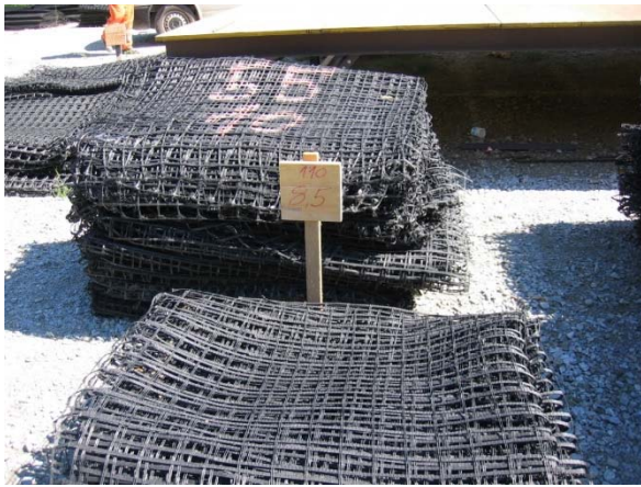
Fig. 9 folded and palletized geogrids
