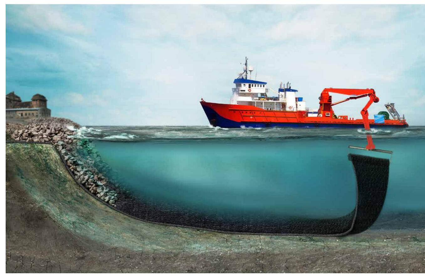
Active Geo-Composites consist of an amendment, or multiple amendments, sandwiched between two geosynthetic layers. These Geo-Composites allow accurate placement of amendments with low densities that could otherwise become suspended during placement.
