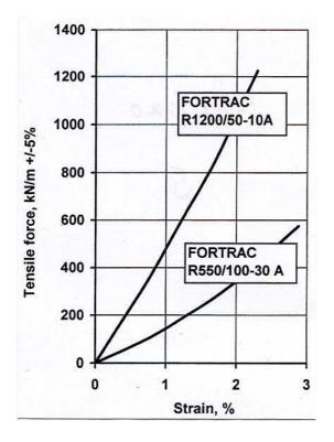
Figure 5. Stress-strain curves (short-term) of the aramid geogrids for the Böschistobel landfill
