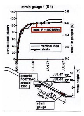
Figure 6. Typical measurement results from a cross-section at the Böschistobel landfill
