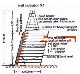
Figure 12. Cross-section of the geogrid reinforced retaining wall at Unterkaka Logistics Centre with PVA-geogrids
