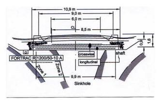
Figure 1. Bridging a sinkhole on the Federal Road B 180: overview of the problem
