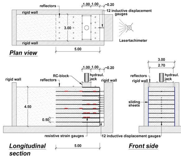
Figure 4. Test set-up and instrumentation of a full scale geogrid reinforced bridge abutment loading test (Alexiew [1]).
