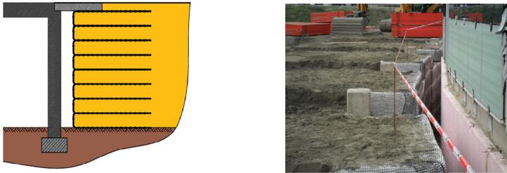
Figure 2. Geogrid-reinforced soil block behind walls as earth pressure relief.
