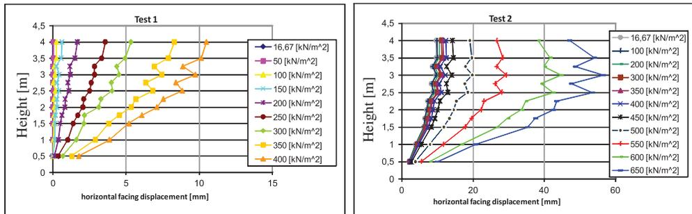
Figure 6. Horizontal facing displacement for load test 1 and 2 (not all load steps are shown).
