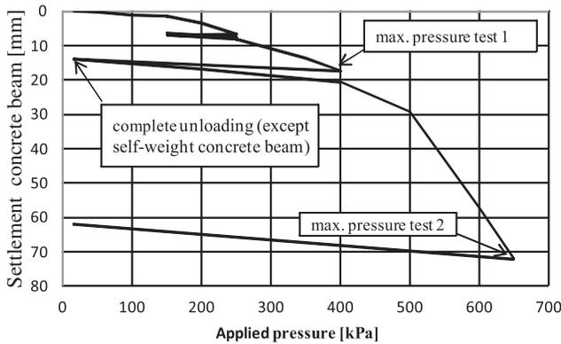
Figure 5. Settlement of the concrete block during the loading test 1 and 2.
