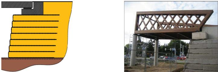
Figure 3. GRS as directly loaded bridge abutment.
