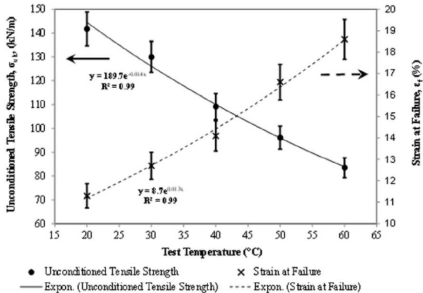
Figure 4 – Relationship between strength and strain for increasing temperatures (Kasozi et al)
