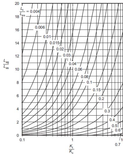
Figure 2 - Dimensionless length in tension,  $L_t/L_{es}$  against stiffness in ratio  $K_t/K_c$  and ratio of exposed length of geosynthetic layer to exposed length of placed cover soil layer,  $L_{eg}/L_{es}$  (Liu and Gilbert, 2005).
