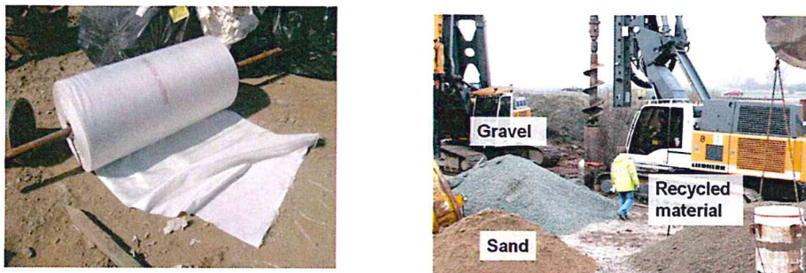
Fig. 3. Typical woven seamless encasement as delivered to the site before installation (left) and different fills for GEC in a field trial (right).
