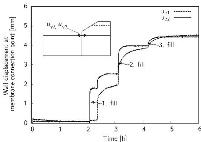
Figure 6. Horizontal wall displacement over time measured at the connection point of the tension membrane to the vertical wall (positive values represent an outward movement).
