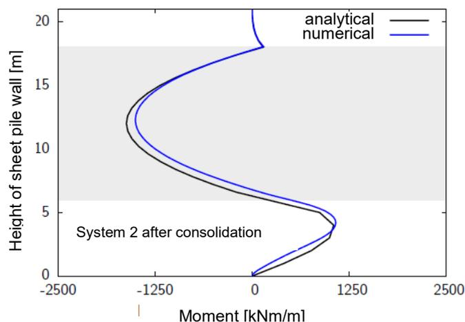
Figure 11. Bending moment of the sheet pile wall over the height. The grey area marks the soft soil layer.
