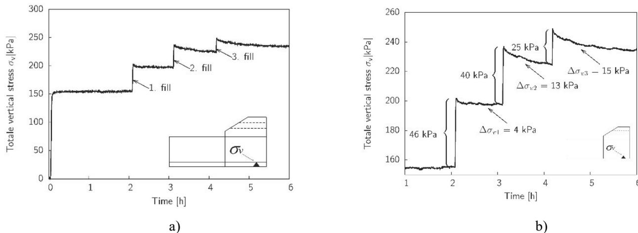
Figure 4. Total vertical pressure over time measured in the drainage layer at the bottom of the model over time for the full range (a) and zoomed in to analyze the different load steps (b).
