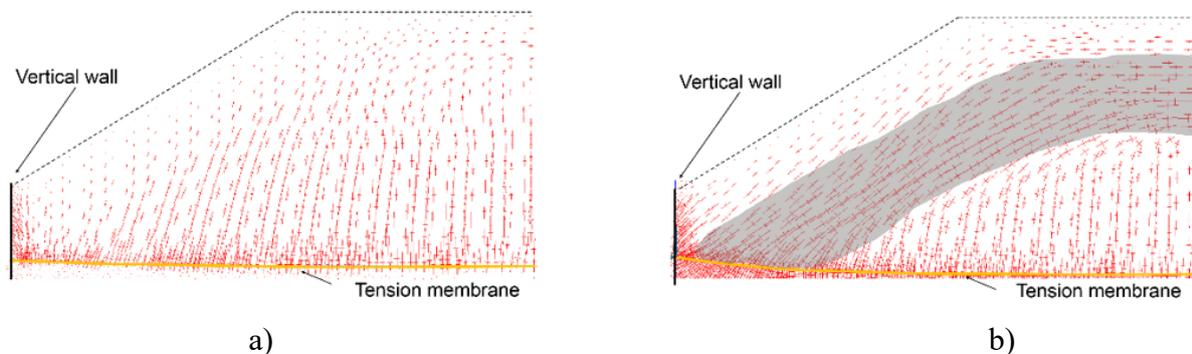
Figure 7. Principal stresses within the embankment body before (a) and after consolidation (b).
