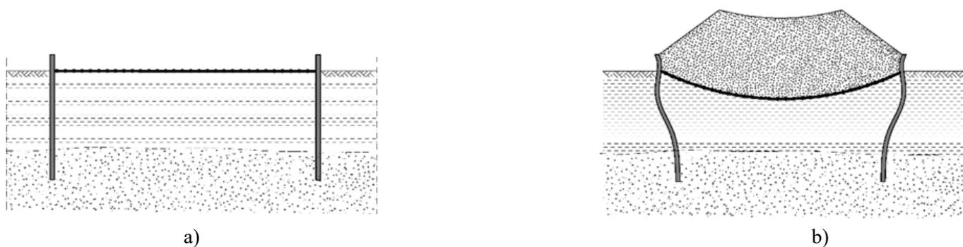
a) Figure 1. System as installed (a); loaded and deformed system (b)
