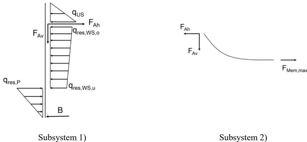
Figure 9. The system is split into two subsystems for design purpose. ( $q_{us}$  = resulting loading on the sheet wall protrusion;  $F_{av} / F_{ah}$  = vertical and horizontal connection forces of the tension membrane;  $q_{res,WS,o} / q_{res,WS,u}$  = resulting loading on the shear wall within the soft soil layer at the top and bottom;  $q_{res,P}$  = resulting loading on the sheet pile wall within in the firm foundation layer;  $B$  = substitution force)
