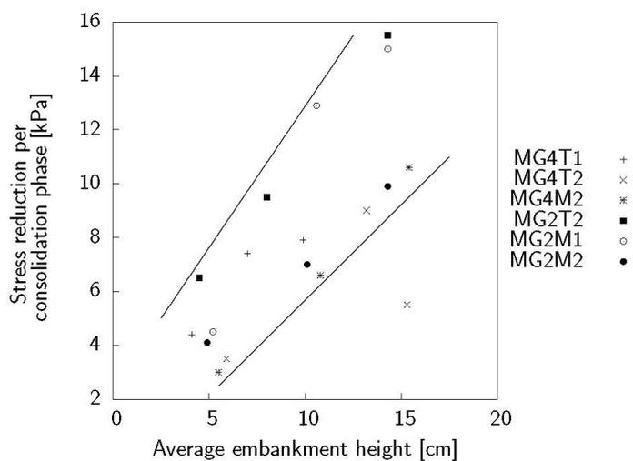
Figure 5. Decrease of total vertical pressure over average embankment height (results of different combinations of tensile stiffness of the geotextile and thickness of model wall; MG = Membrane Foundation; 4 = 4 mm and 2 = 2 mm model wall thickness; T = Geogrid Polyester, M = Geogrid Polyvinylalcohol, last number either test no. 1 or test no. 2).
