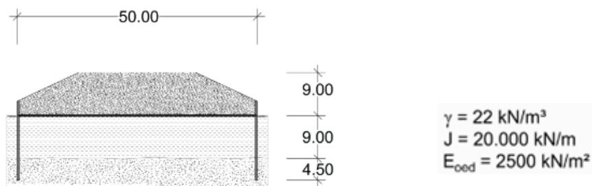
Figure 10. System configuration for comparative calculation between the developed approach using the design charts and numerical methods ( $\gamma$  = unit weight embankment,  $J$  = tensile stiffness membrane,  $E_{oed}$  = oedometric modulus soft soil)
