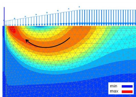
Figure 8. Rotational movement (most probable failure mechanism) within the soft soil beneath the embankment.
